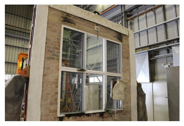
Photograph 7 - Exposed face of the specimen at the completion of testing
