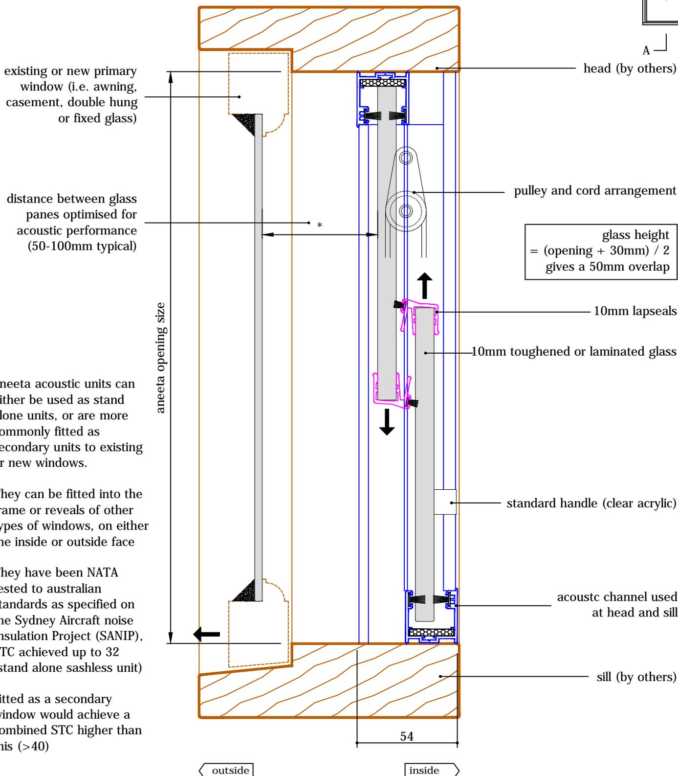
aneeta acoustic units can either be used as stand alone units, or are more commonly fitted as secondary units to existing or new windows.
