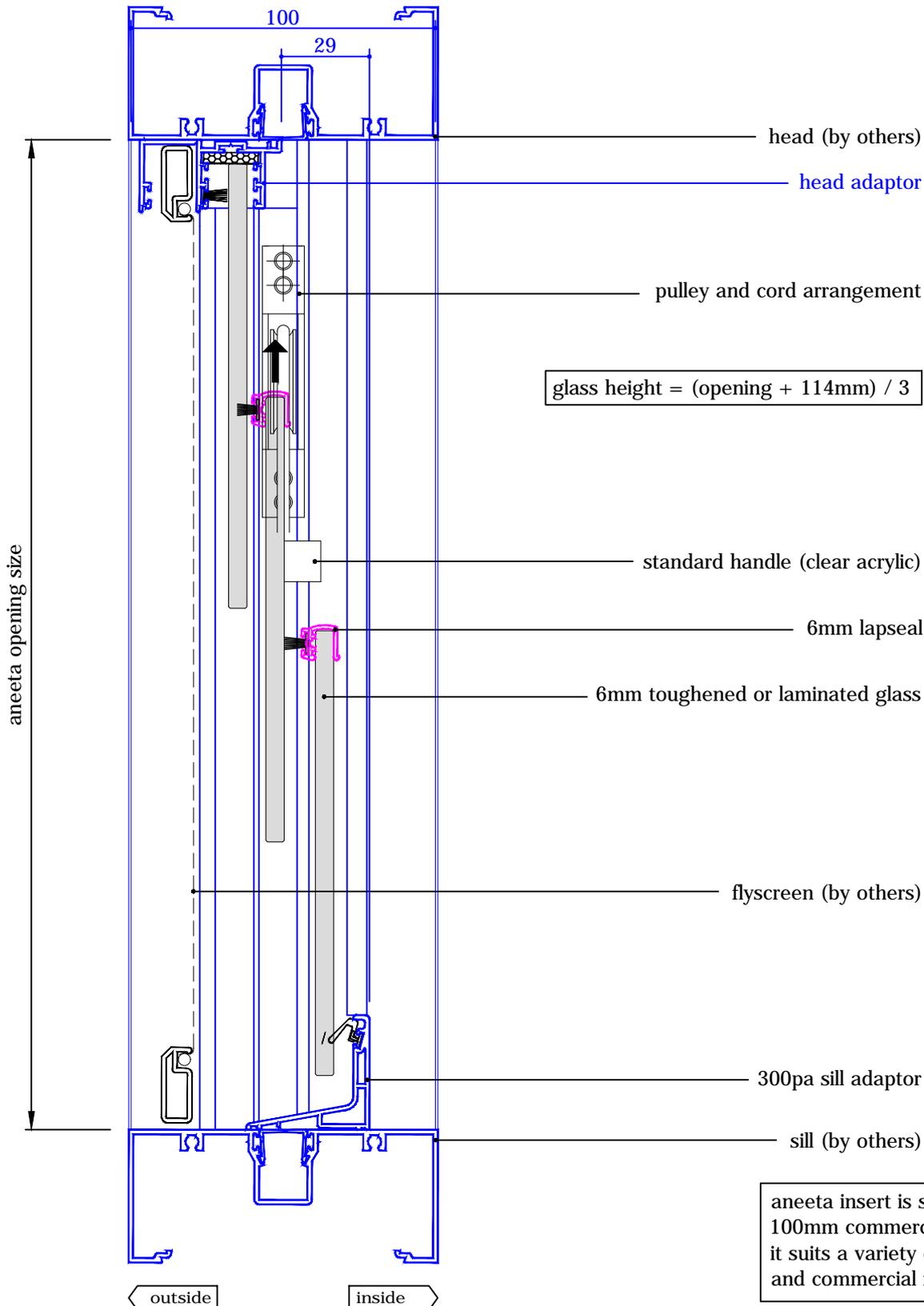
$$\text{glass height} = (\text{opening} + 114\text{mm}) / 3$$
