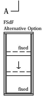
aneeta insert is shown here in 100mm commercial framing but it suits a variety of residential and commercial frame types
