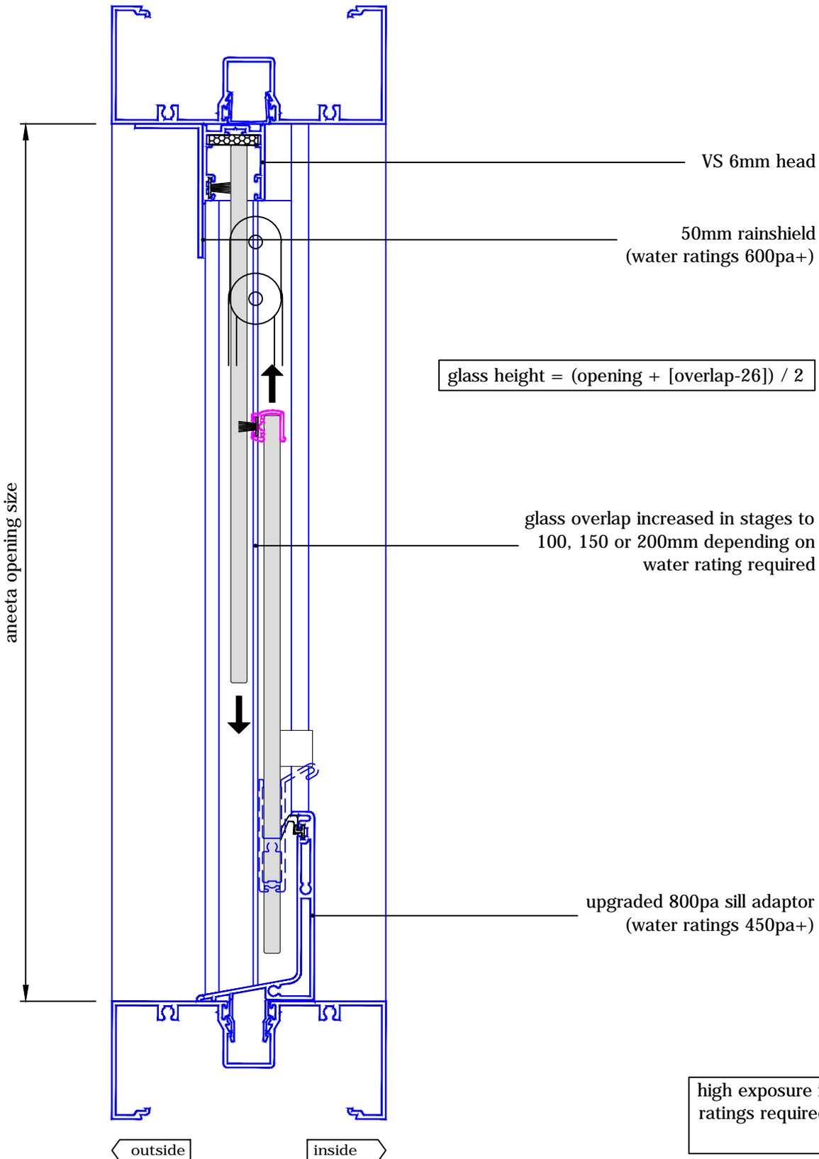
high exposure is where water ratings required are 450pa or higher
