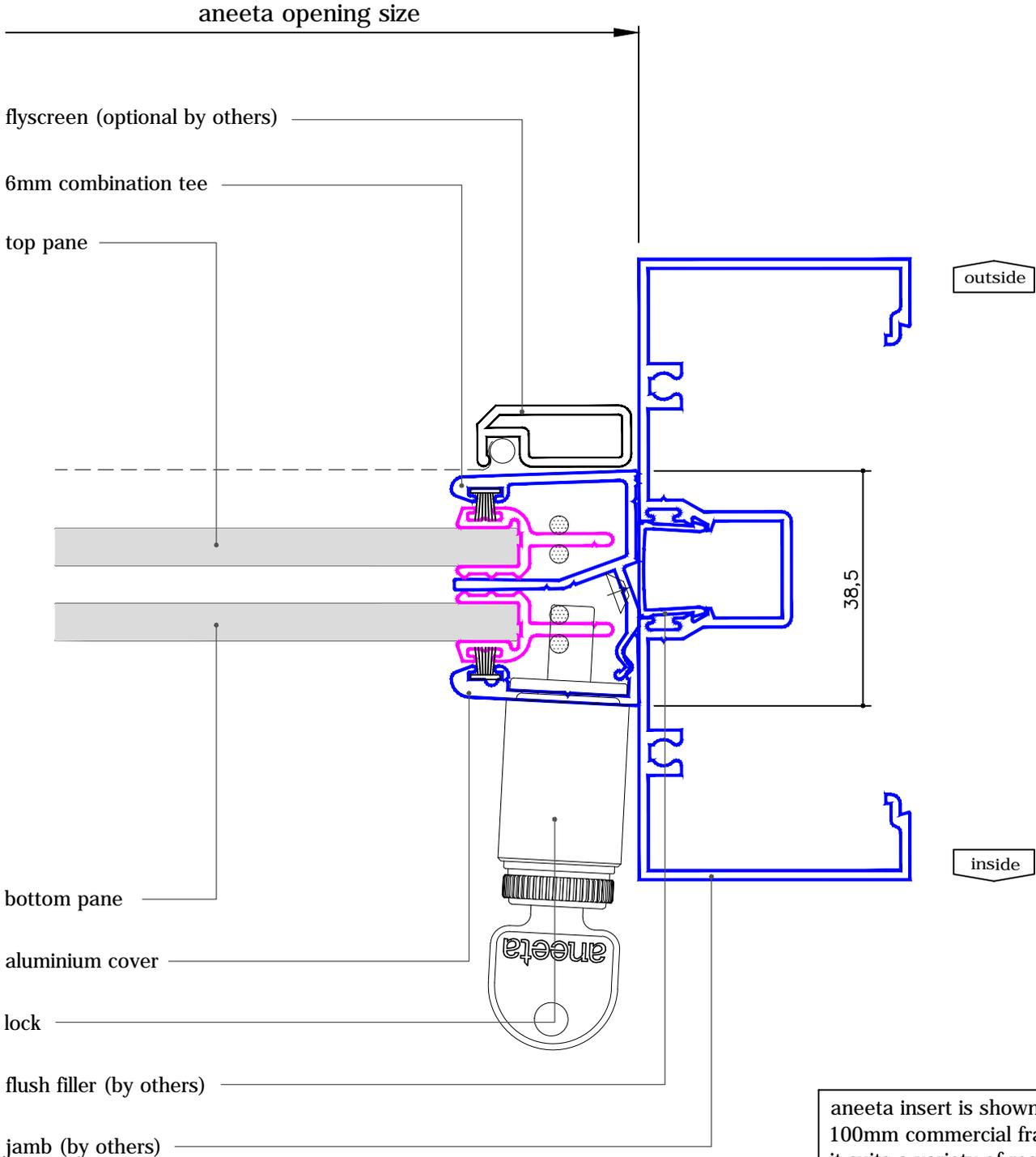
aneeta insert is shown here in 100mm commercial framing but it suits a variety of residential and commercial frame types
