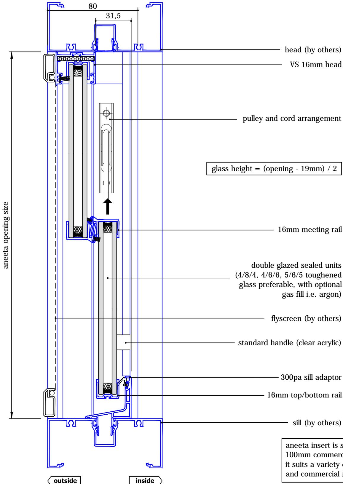
aneeta insert is shown here in 100mm commercial framing but it suits a variety of residential and commercial frame types
